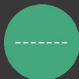
Aspherical | The glass is curved in two points to further extend the field of view. Glass which is aspherical in nature is usually finished with a solid or dotted black line situated towards furthest edge.
